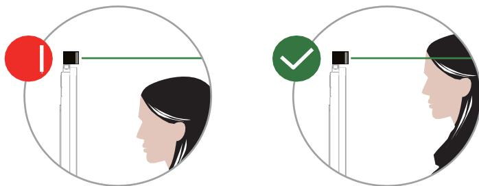
Note: If your terminal is a wrist temperature measurement terminal, please come closer, raise your wrist and then make your inside wrist point at the temperature measurement sensor (1~5cm away from the TM sensor).
