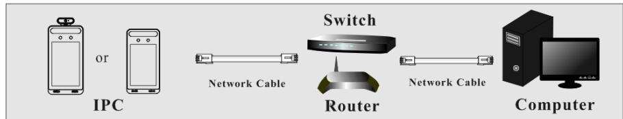
① Make sure the PC and IP-Cam are connected to the LAN and the IP-Tool is installed in the PC from the CD.
