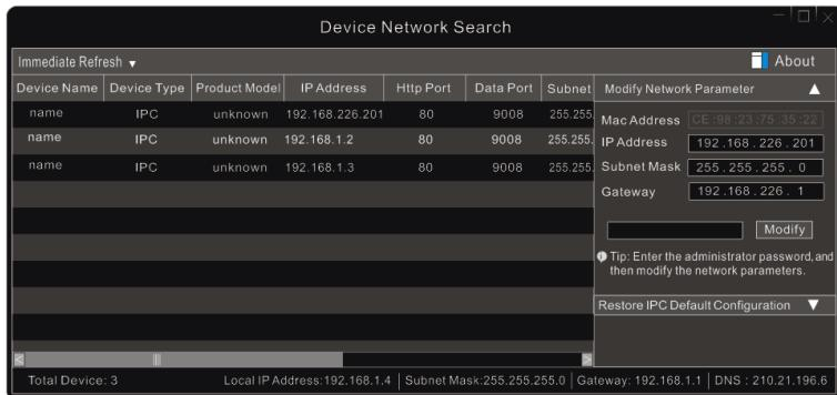
③ Modify the IP address. The default IP address of this camera is 192.168.226.201. Click the information of the camera listed in the above table to show the network information on the right hand. Modify the IP address and gateway of the camera and make sure its network address is in the same local network segment as the computer's. Please modify the IP address of your
