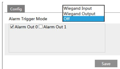
**Alarm Trigger Mode:** Wiegand Input, Wiegand Output or Off can be selected. If the card reader is connected to the Wiegand interface, please select “Wiegand Input”. If the access controller is connected to the Wiegand interface, please select “Wiegand Output”. You can also select the alarm output as needed.
