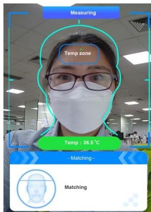
The system will measure the temperature and compare the captured face at the same time as shown below.
