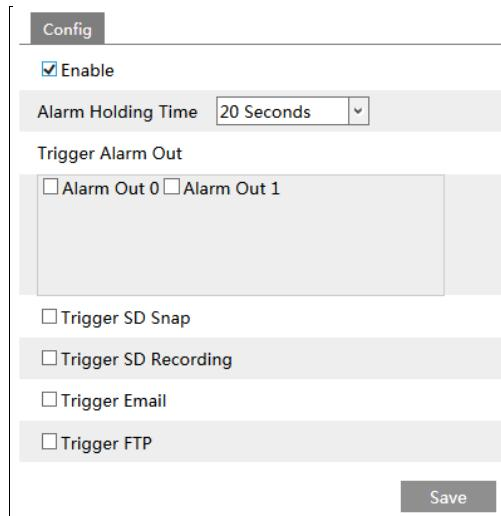
Enable “Tampering Alarm” and then set the alarm holding time and alarm trigger options. The setup steps of the alarm trigger options are the same as temperature measurement settings. Please refer to temperature measurement settings chapter for details.
