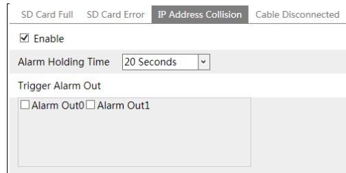
2. Click “Enable alarm” and set the alarm holding time.
