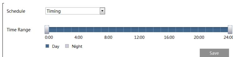
Drag “” icons to set the time of day and night. Blue means day time and blank means night time. If the current mode of camera parameters is set to schedule, the image configuration mode will automatically switch between day and night according to the schedule.
