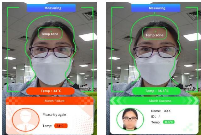
When the captured face is not added to the face database or the similarity is lower than the pre-defined value, it will display “Match Failure” and the box will turn red.
